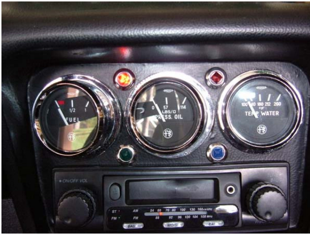
Spider Center Instrument Panel. Note Fuel Low Pressure Warning Light Illuminated. Fig 4
