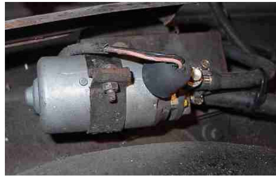
'69-'74 2-port Pump Installation (right axle area). Fig 1
