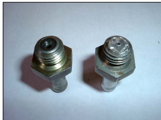
Outlet Restrictors. Left one is stock (3/32"). Right one has been soldered-in and re-drilled with a 1/16" drill.
